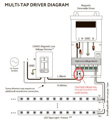
† Install a compatible magnetic low voltage dimmer switch. See dimmer switch manufacturer installation guide for complete wiring instructions.
